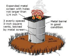
Ground cleared down to mineral soil or gravel at least 10 feet on each side of incinerator
